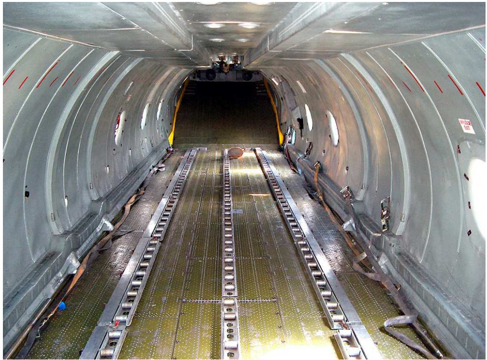
Roller floor in cargo compartment
